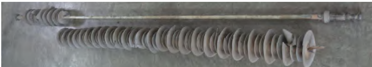
Figure 2.14: Silicone rubber housing removed from failed SRI-2
