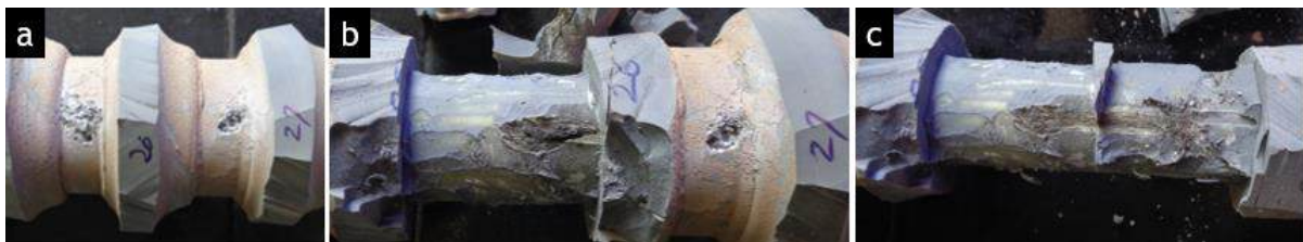
Figure 2.36: a) Punctured sheath, b) composite rod under first puncture and c) composite rod under the second puncture
