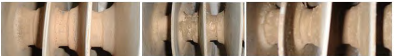
Figure 2.18: Silicone rubber sheath mostly covered with dust and algae but no punctures
