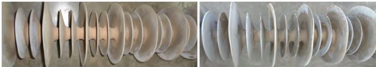
Figure 2.23: As received working insulator (SRI-4) received for analysis
