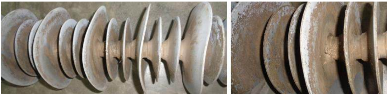
Figure 2.17: Most of the silicone rubber housing was covered with algae
