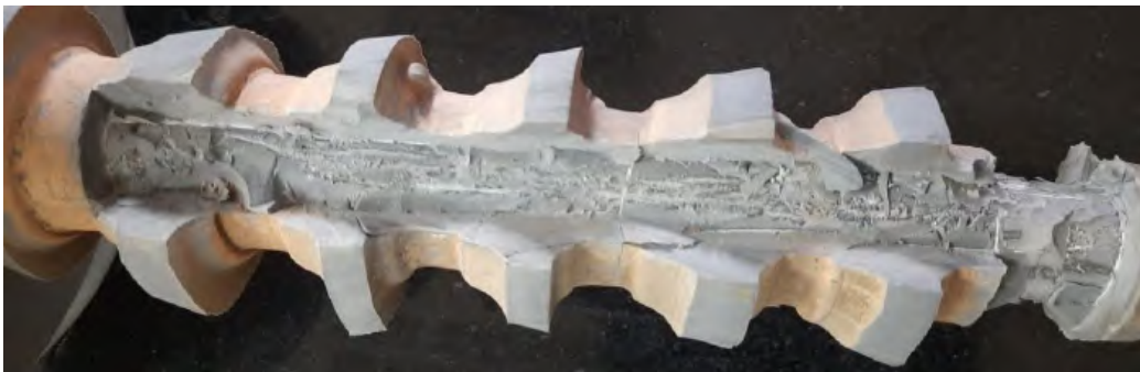
Figure 2.20: Stripe test on SRI-3, the interface was found good
