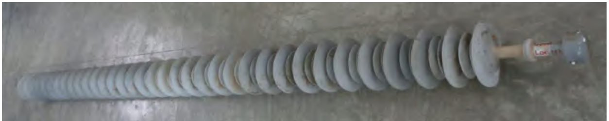
Figure 2.16: As received working insulator (SRI-3) received for analysis
