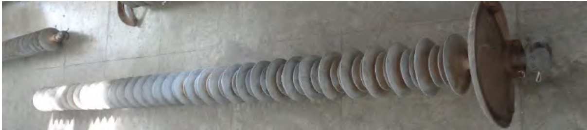
Figure 2.22: As received working insulator (SRI-4) received for analysis
