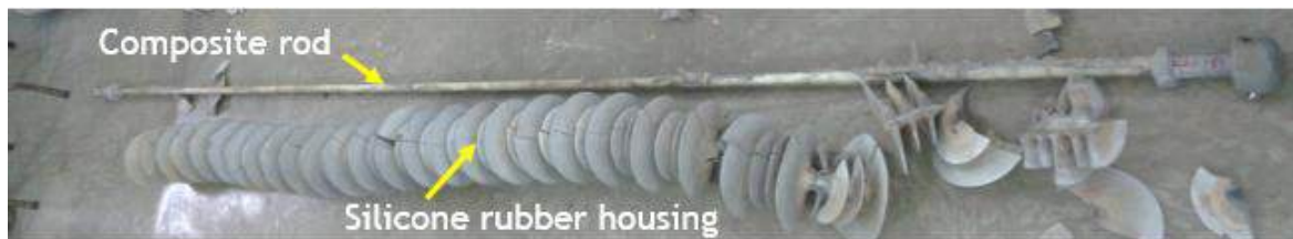
Figure 2.5: Failed insulator silicone housing separated from the composite rod
