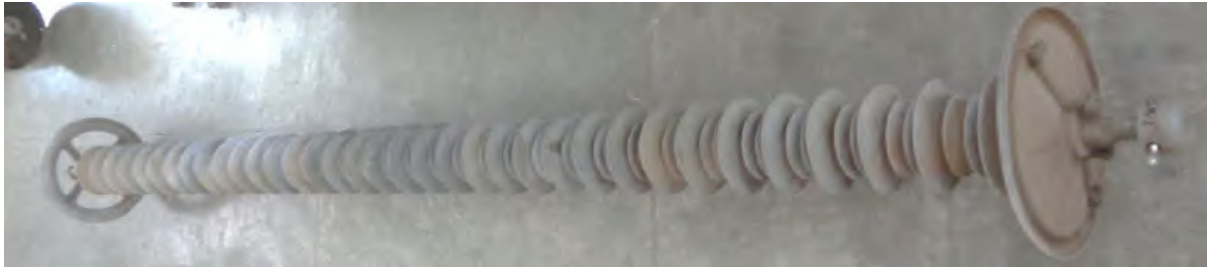
Figure 2.32: As received working insulator (SRI-5) received for analysis
