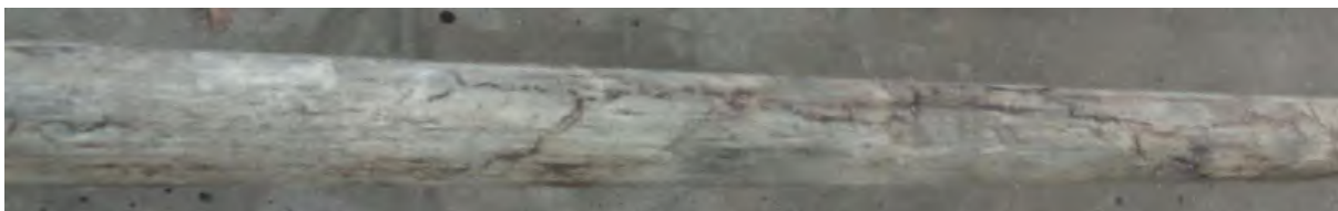
Figure 2.15: Tracking marks were found on entire length of composite rod from SRI-2
