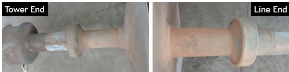
Figure 2.34: Silicone rubber seal at tri-junction with metallic end fittings
