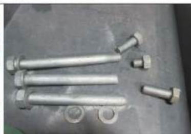
Bolt and nut Ultimate Strength Test
