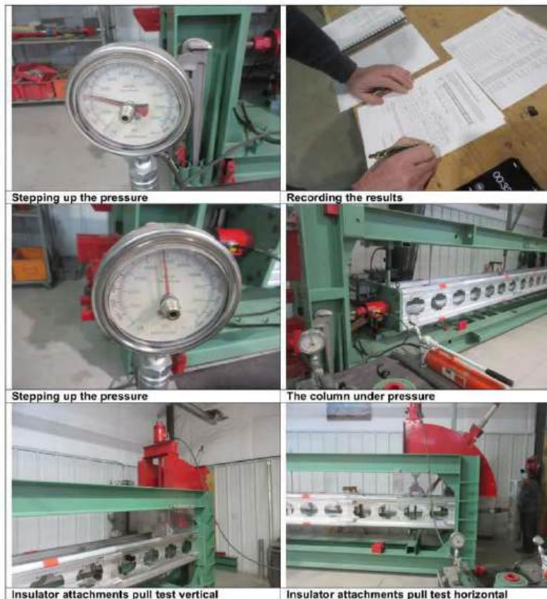
Insulator attachments pull test vertical
