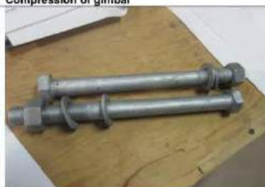
Bolt and nut Ultimate Strength Test
