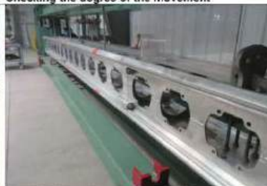
Combined bending and compression test
