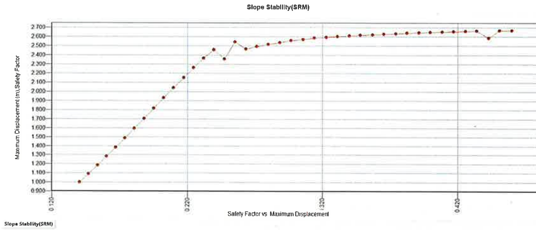
Figure 10. The FoS of the slope as per MIDAS GTS NX analysis with FoS value as 2.66
