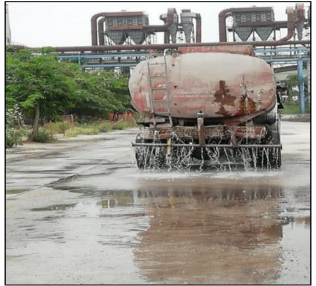
FIGURE 7: WATER SPRAY THROUGH TANKER IN ASH DYKE AREA
